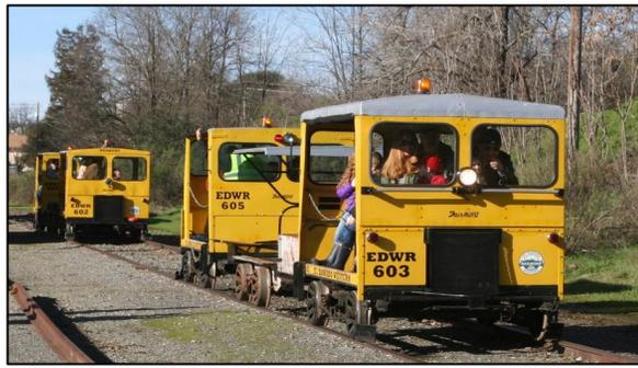
**Speeder Cars**—also known as “Gang Cars,” “Inspection Cars” or “A-Cars”—were rail vehicles used to transport maintenance workers, track inspectors and assorted railroad ruffians for over 100 years from the late 1880s to the early 1990s. Unique in their own right, the gasoline -powered Speeder Cars have developed quite a following of devoted fans.
